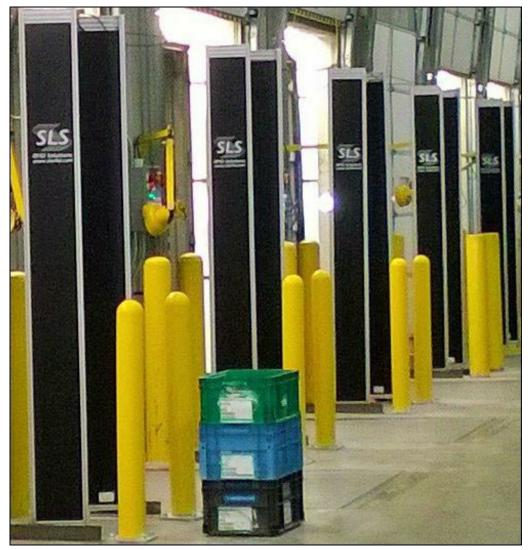
At each side of its dock doors, Johnson Controls bolted a smartPORTAL to the floor.
