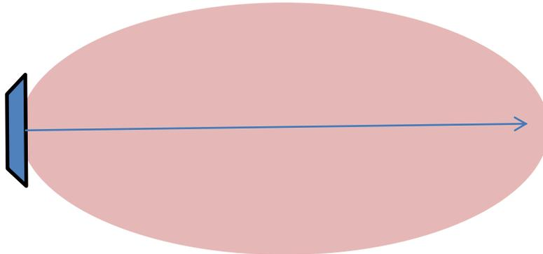
*“Spotlight” pattern of a typical UHF RFID patch antenna.*
