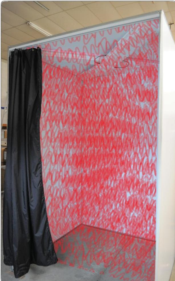
with a metalized curtain, the Surround Portal takes advantage of the highest allowable power density to provide optimal RFID read performance.
