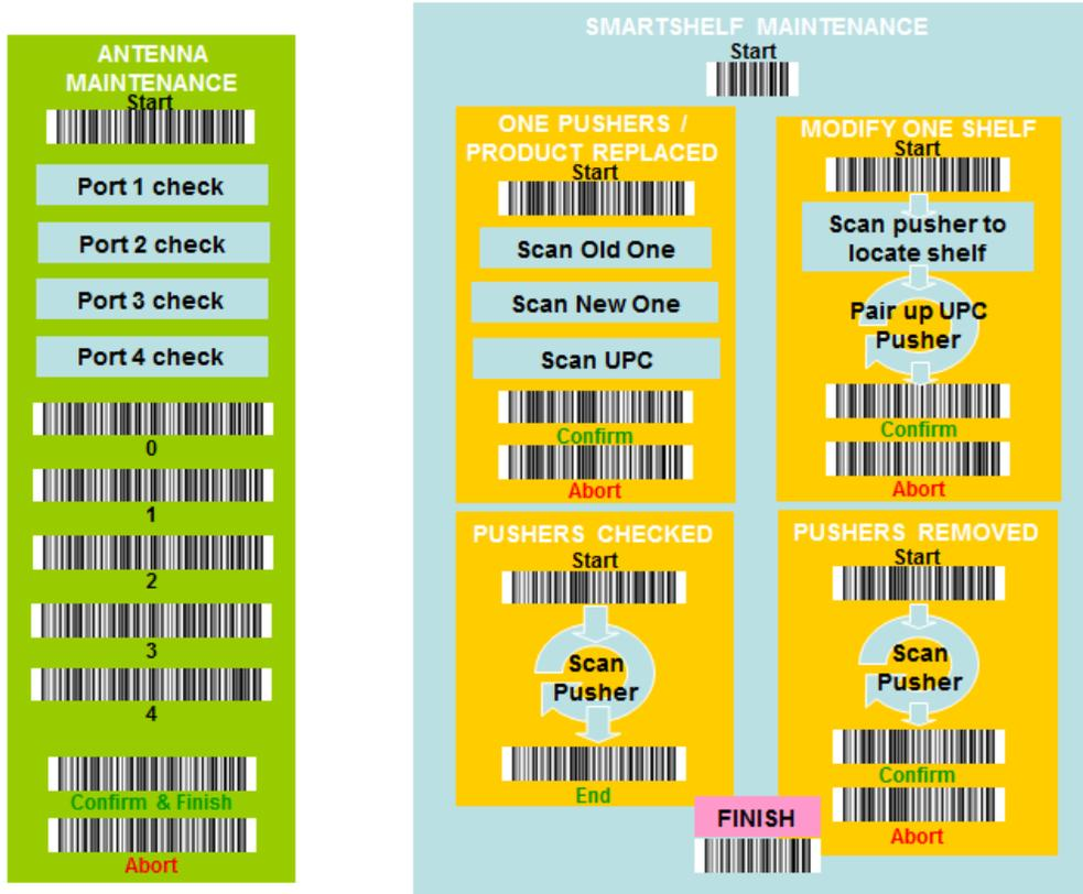
Figure 3.1 Bar code scanner flow chart and commands to do Smart Shelf maintenance.
